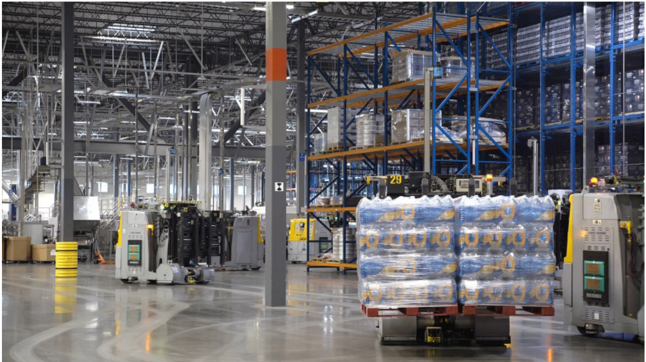
Dual pallet movement with the model CB30 Dual Drive LGV. Image courtesy of E80
