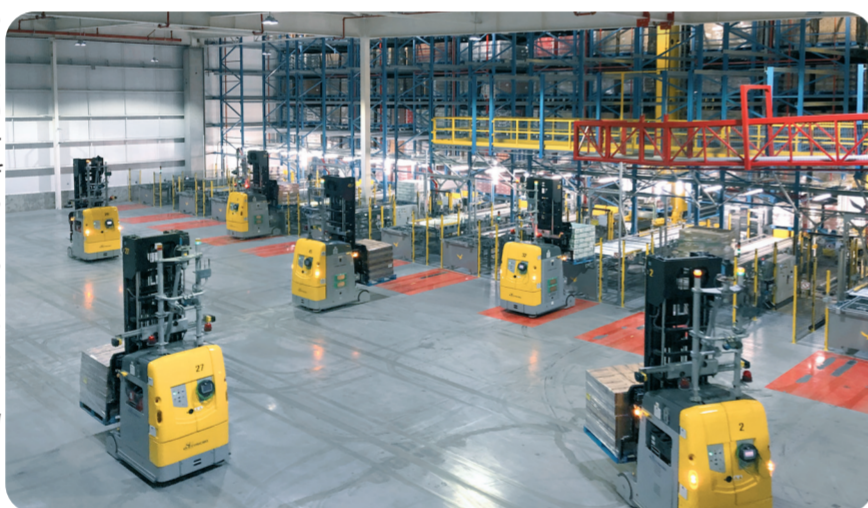
Integrated management of a high-density automated warehouse with laser-guided vehicles
