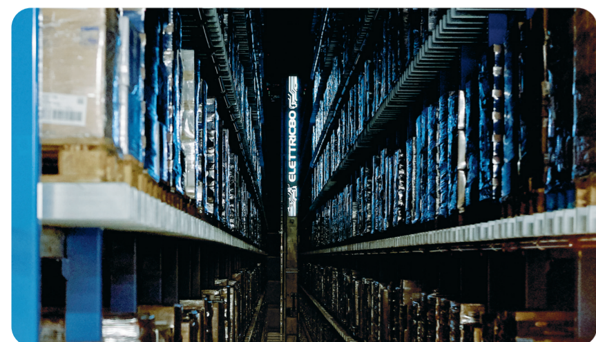
AS/RS Stacker Crane high-density automated warehouse
